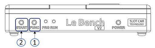
The PRG and RUN LEDs flash 3 times and then turn off, indicating the stop of the Bench V2.
