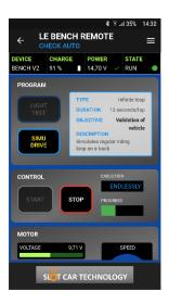
The **SIMU DRIVE** test verifies the vehicle's dynamic behavior by simulating driving on the track and performing a succession of laps.
